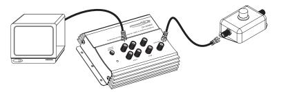
Insert the variable attenuator before the amp. (If you have splitters between the amp and TV, that's OK.) By *increasing* the attenuation, you are *decreasing* the signal that reaches the amp. If you find that the herringbone patterns disappear, then your problem is an overdriven amplifier.
