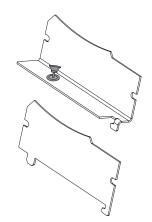
Your DA-506BID is supplied with extra mounting ears. These allow the DA-506BID to be mounted in any OpenHouse<sup>™</sup> structured wire grid system.
